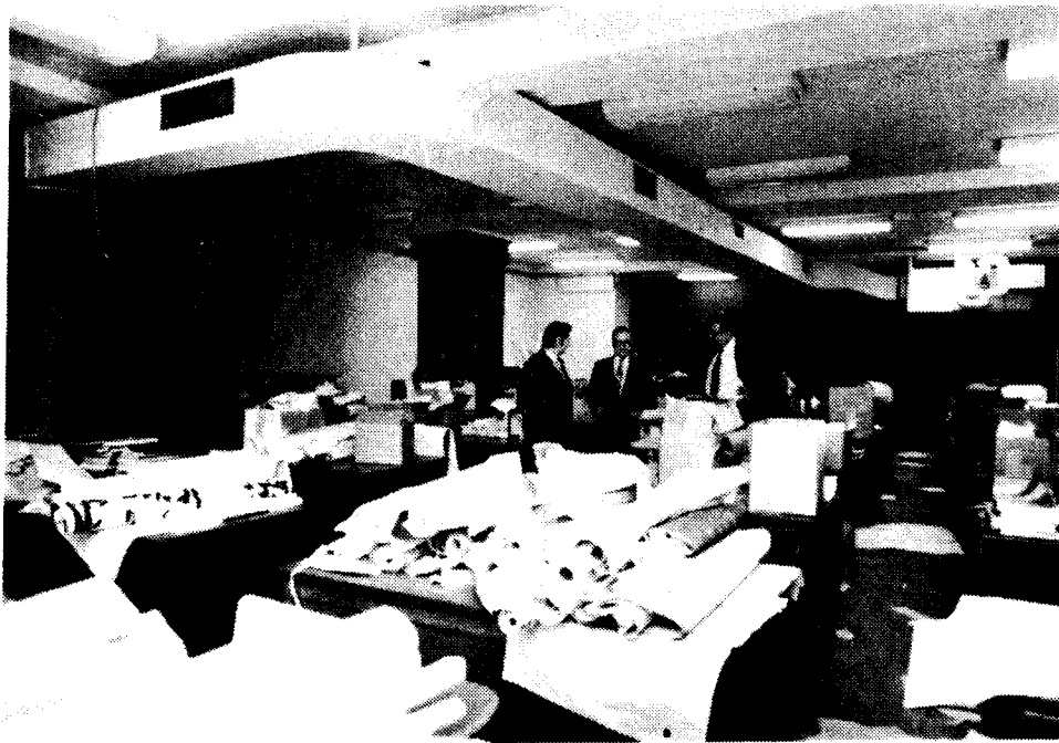
No. 36 - Completion of build-up of fire load in the 7th floor, west wing area for test No. 1. Approximately 6.3 lbs. per sq. ft. of floor area.
