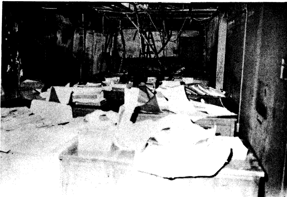
No. 82 - Test No. 4 fire load in place. Note burned out area of fire for Test No. 2 in background.
