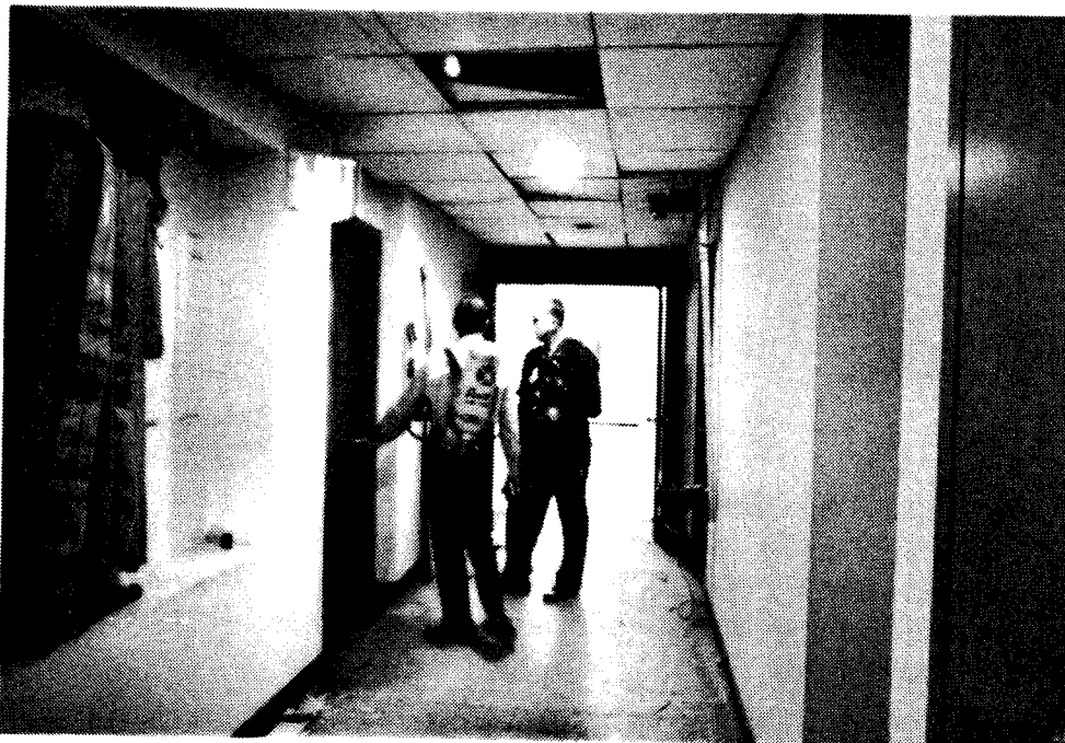
No. 33 - Establishing stair pressurization level in test stairwell during cold smoke tests. Note differential pressure gauges in use.
