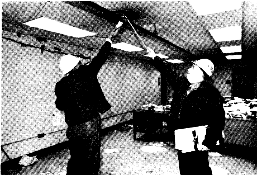
No. 55 - Fire load for Test No. 2 in background. Fusible link in water spray head being removed. Note instrumentation wiring and tubing along upper wall.
