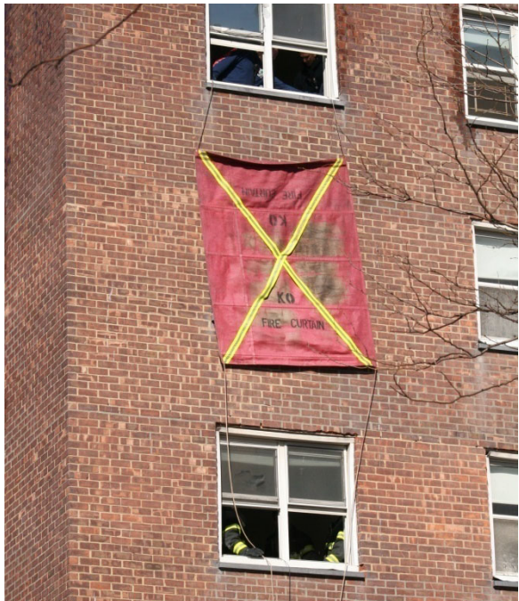
Figure 1.8-6. Wind Control Device Deployed
