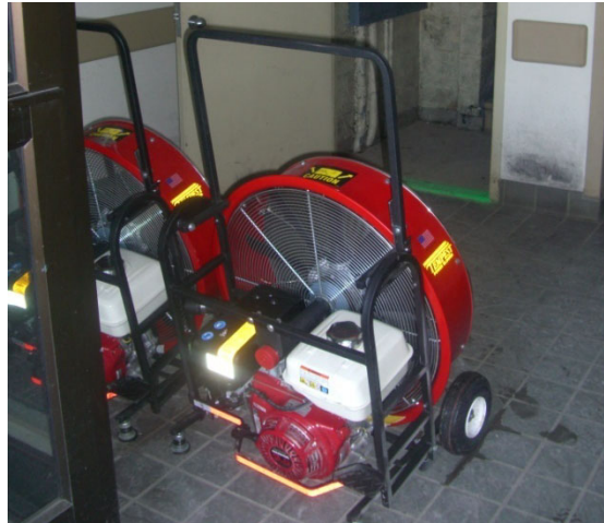
Figure 1.7-2. Rear View of PPV Fans
