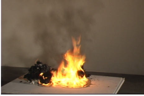
Figure 3.2-14. Trash container 2, 400 s after ignition
