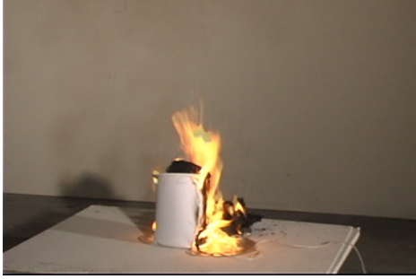
Figure 3.2-12. Trash container 2, 300 s after ignition
