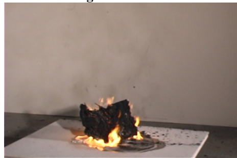
Figure 3.2-8. Trash container 1, 600 s after ignition
