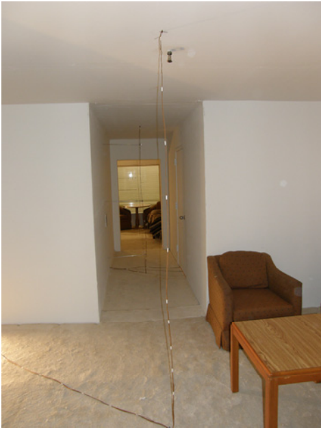
Figure 4.1.3-2. Thermocouple arrays along center line of structure looking from east to west.
