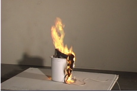
Figure 3.2-11. Trash container 2, 200 s after ignition
