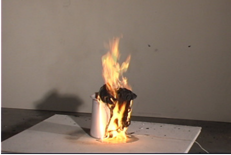
Figure 3.2-3. Trash container 1, 200 s after ignition
