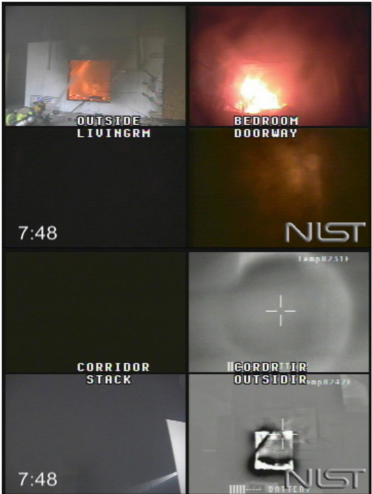
Figure 5.8.1-13. Experiment 8, indirect suppression stopped, 468 s after ignition.
