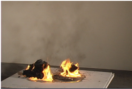
Figure 3.2-16. Trash container 2, 600 s after ignition
