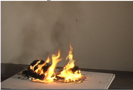
Figure 3.2-15. Trash container 2, 500 s after ignition
