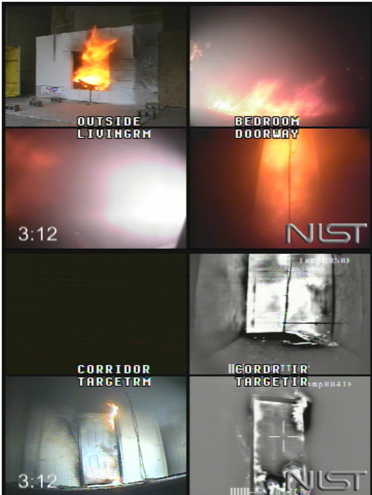
Figure 5.6.1-6. Experiment 6, corridor flames, 192 s after ignition.
