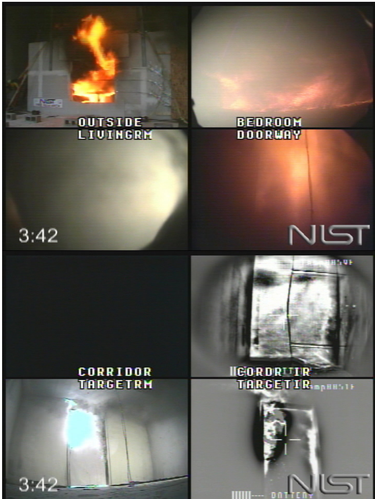
Figure 5.3.1-6. Experiment 3, corridor flames, 222 s after ignition.
