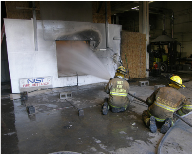
Figure 4.3.3-3. Fog stream discharged into window opening.
