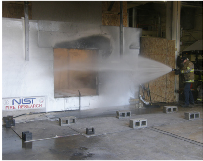
Figure 4.3.3-2. Fog stream discharged across window opening.
