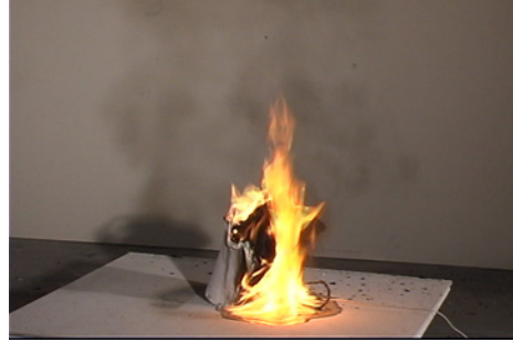
Figure 3.2-4. Trash container 1, 300 s after ignition
