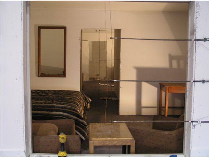
Figure 4.1.3-3. Bi-directional probe array in west window.
