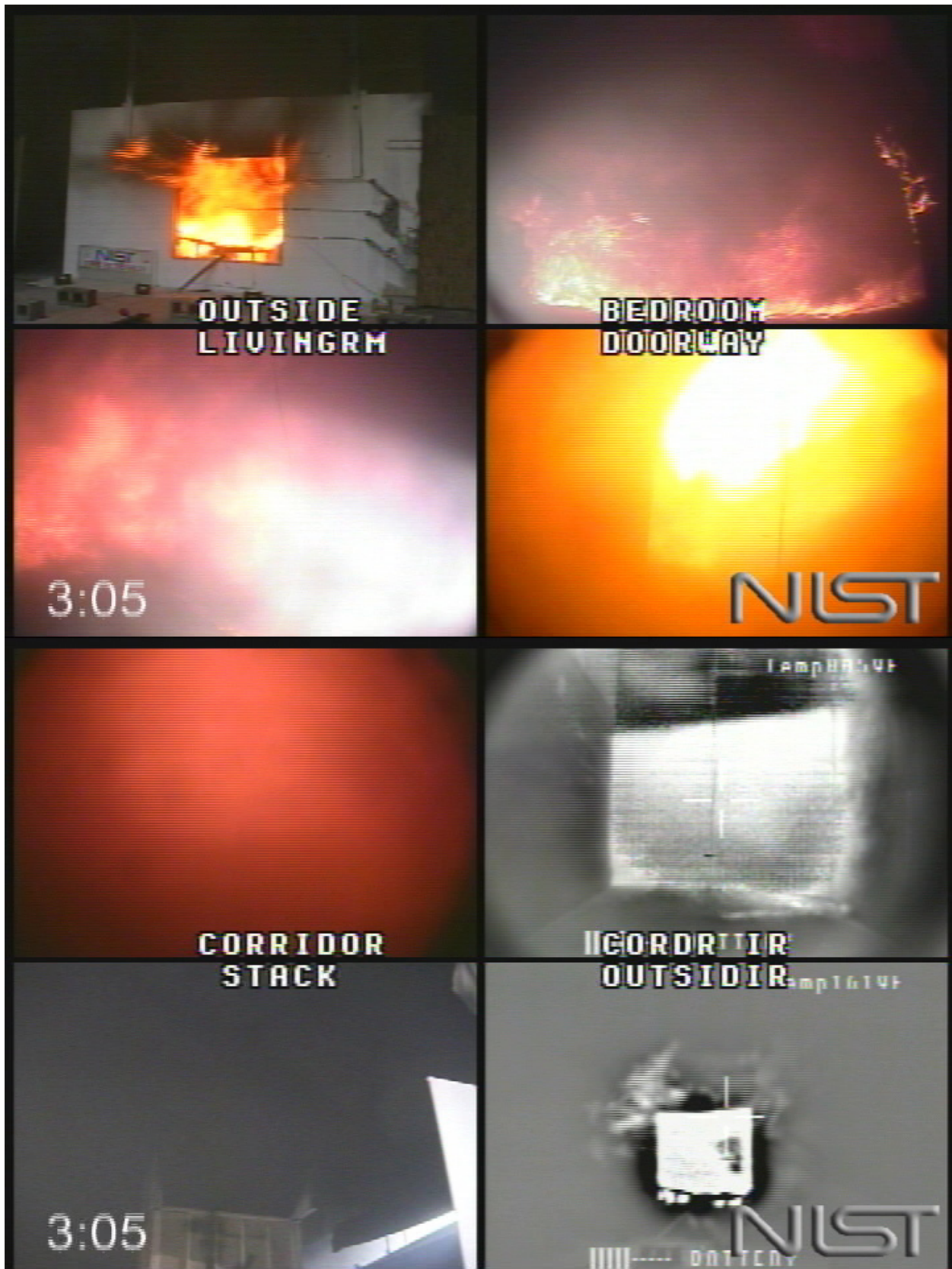
Figure 5.8.1-6. Experiment 8, corridor flames, 185 s after ignition.
