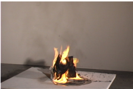
Figure 3.2-7. Trash container 1, 500 s after ignition
