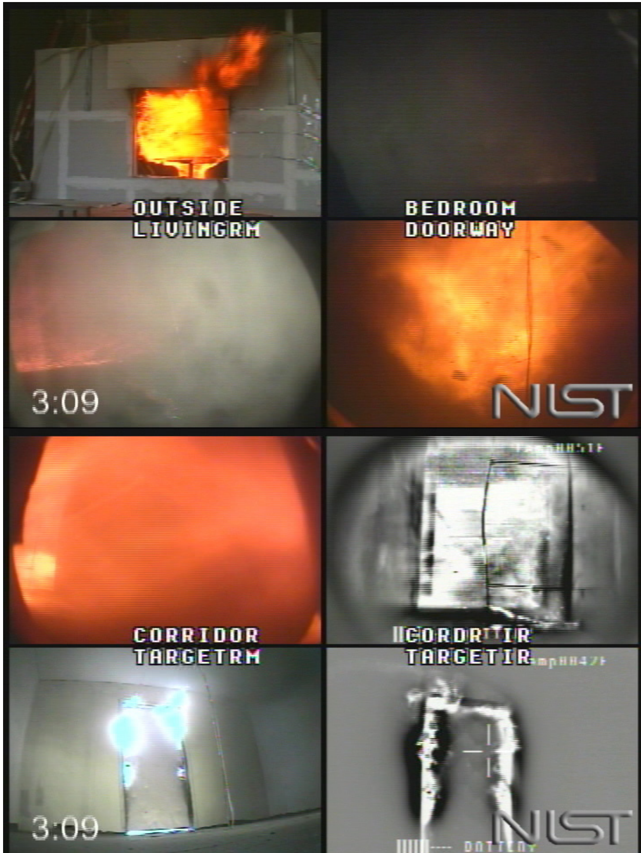
Figure 5.2.1-5. Experiment 2, corridor flames, 189 s after ignition.
