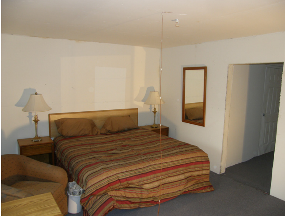
Figure 5-1. Photograph of the placement of the trash container fuel package ignition source.
