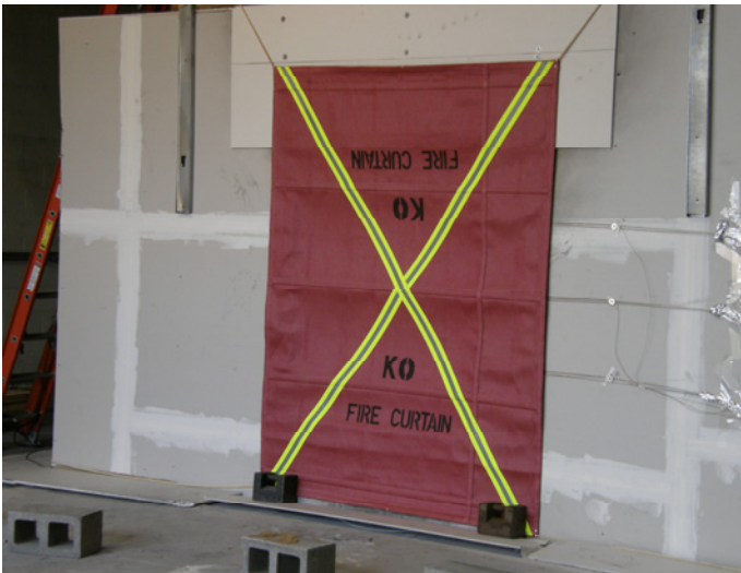
Figure 4.3.2-1. Small WCD deployed over window opening.
