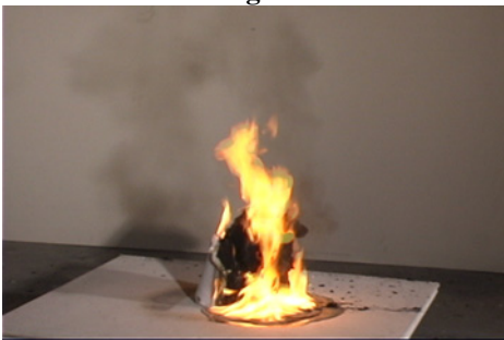
Figure 3.2-5. Trash container 1, 400 s after ignition
