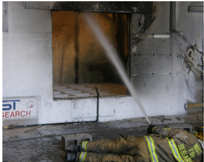
Figure 4.3.3-4. Solid stream discharged into window opening.
